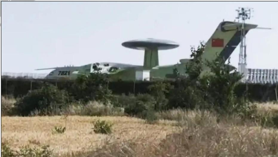
New imagery has emerged of China's new heavyweight airborne early warning and control (AEW&C) platform, the KJ-3000. Based on the four-jet Y-20 cargo plane, the KJ-3000 is part of a fast-expanding and diversifying fleet of Chinese AEW&C aircraft, which also includes multiple iterations based on the four-turboprop Y-9 series of airlifters.
