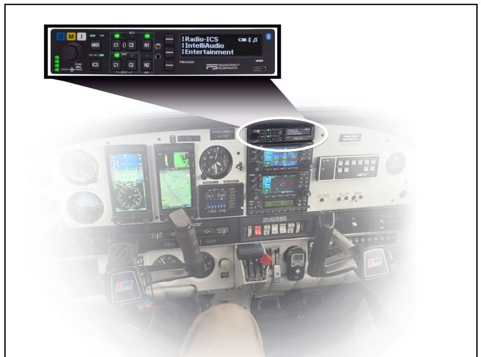
An installed PS Engineering PMA450A audio panel is shown. (Photo courtesy of PS Engineering.)
