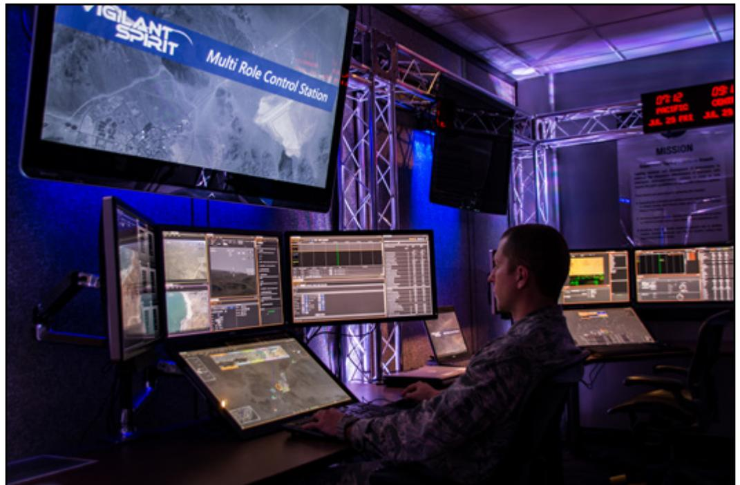
*Captain Anthony Castello views the Vigilant Spirit Control Station at Wright-Patterson Air Force Base, Ohio. Engineers in the 711HPW's Supervisory Control & Cognition Branch developed the software which allows operators to control multiple UAVs at once. The software package offers multi-role, human-machine teaming and an advanced simulation and training component. It is currently being shared with the multiple companies through information transfer agreements. (Courtesy photo)*
