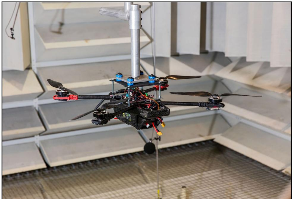
*A small unmanned aerial system undergoes tests in the Acoustics Laboratory at Owens Corning Science and Technology Center in Granville, Ohio. (Photo courtesy of Owens Corning)*
