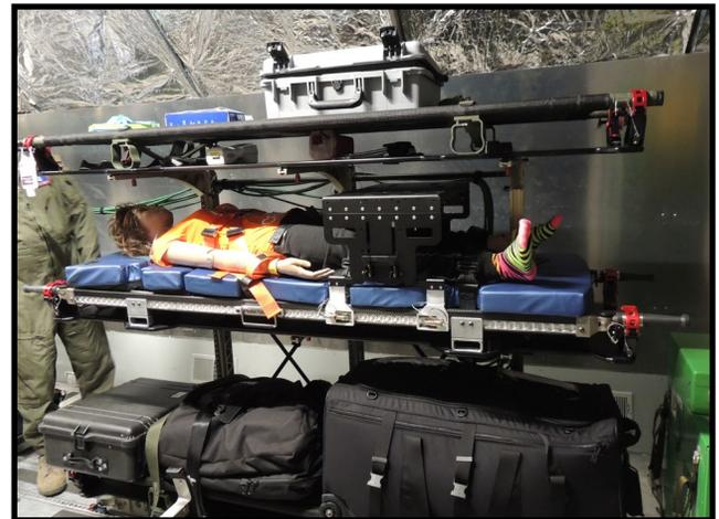
*Cornerstone Research Group’s aeromedical evacuation stretcher is shown during a compatibility test on a KC-135. (Photo courtesy of Cornerstone Research Group.)*
