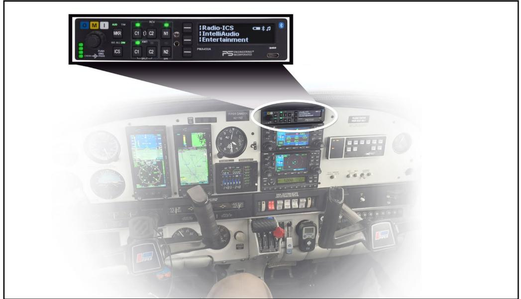
An installed PS Engineering PMA450A audio panel is shown. The audio panel includes an Air Force multi-talker technology licensed by PS Engineering through a patent licensing agreement. (Photo courtesy of PS Engineering.) See story on page 2.
