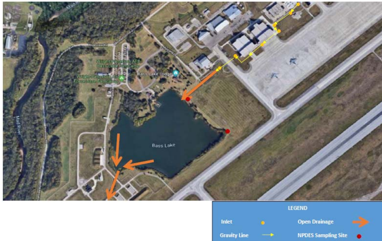
Figure 5. Storm Water Flow for Project Location.
